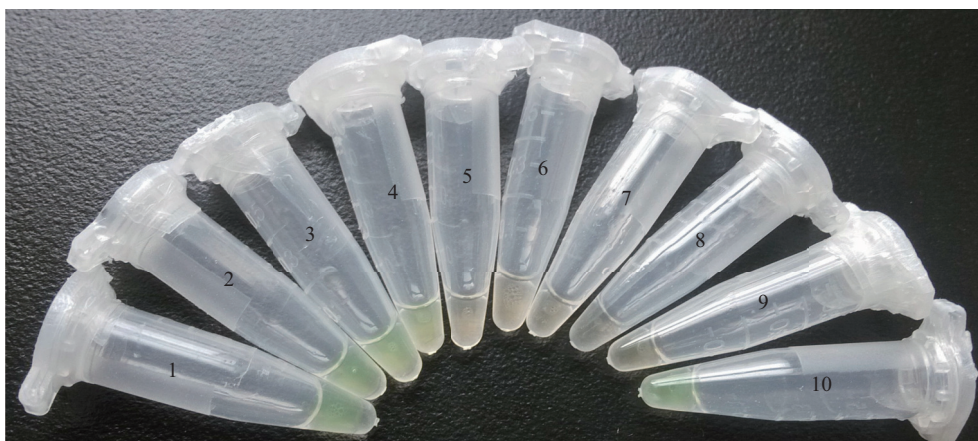
Fig. 4. The sensitivity of LAMP assay by naked-eye examination. Tube 1: 4 \times 10^3 CFU/tube, Tube 2: 4 \times 10^2 CFU/tube, Tube 3: 4 \times 10^1 CFU/tube, Tube 4: 4 \times 10^0 CFU/tube, Tube 5: 4 \times 10^{-1} CFU/tube, Tube 6: 4 \times 10^{-2} CFU/tube, Tube 7: 4 \times 10^{-3} CFU/tube, Tube 8: 4 \times 10^{-2} CFU/tube, Tube 9: negative control, and Tube 10: positive control.
