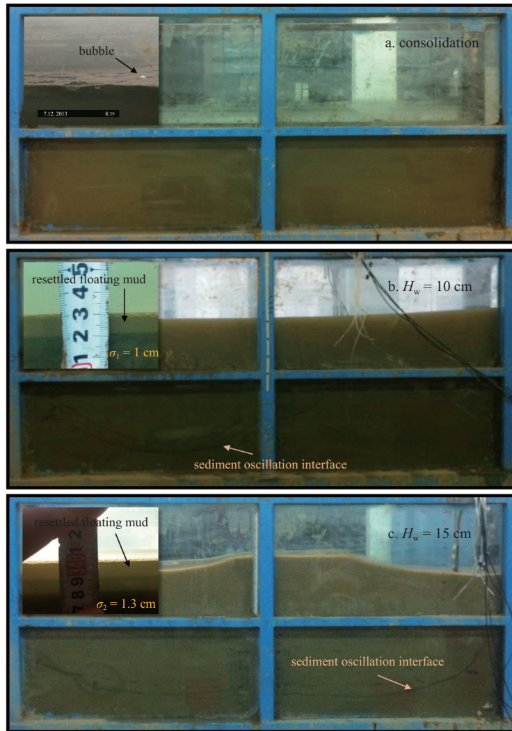
Fig. 3. Side view of the experimental layout. a. In consolidation period before wave action during which tiny bubbles appeared on the seabed surface; b. under 10 cm waves during which seabed shear failure with partial fluidization occurred, after which a floating mud layer of 1 cm in thickness formed; and c. under 15 cm waves during which seabed shear failure with partial fluidization occurred in a larger area, after which a floating mud layer of 1.3 cm in thickness formed.
