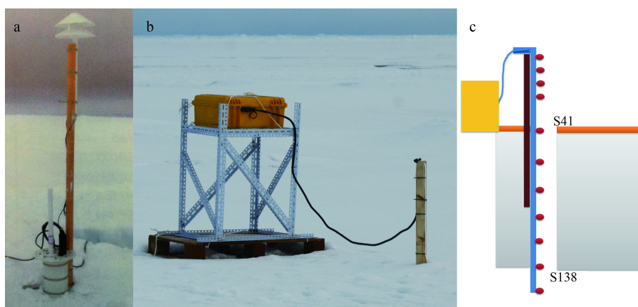
Fig. 2. The Zeno ® and SIMBA (NMEFC02) deployed during CHINARE 2003 (a), and CHINARE 2014 (b); and a schematic illustration of NMEFC02 vertical sensor distribution is given (c).
