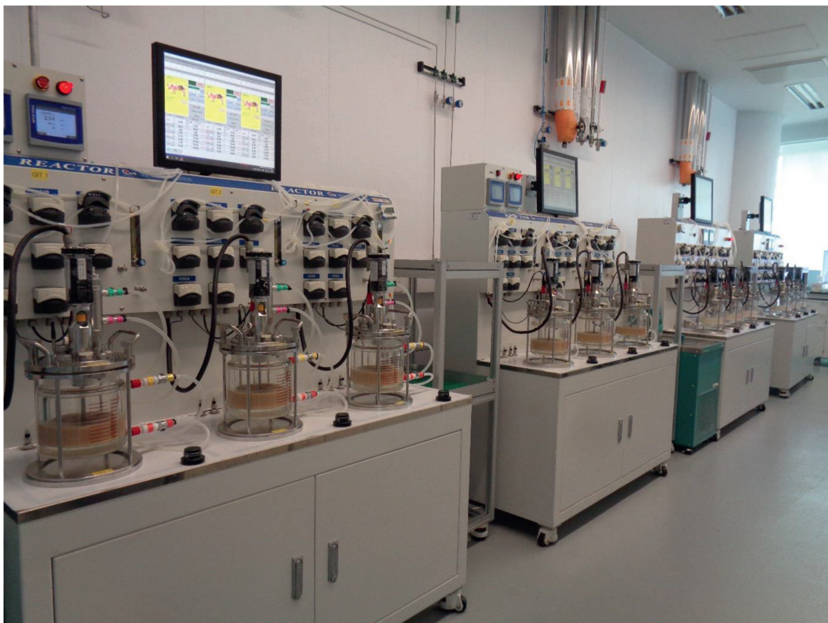
Fig. 2. The artificial gastrointestinal model with 12 digestion chambers (CJ Blossom Park, Suwon, Republic of Korea).
